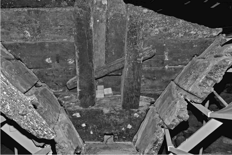
FIGURE 39. Mast support structure of the Shinan ship. Courtesy of the National Maritime Museum of Korea, photo by author.
